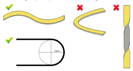
Cable and connector should never be stretched. Also, the LED strip should not be twisted. The LED strip is completely encapsulated and designed for versatile Use. It can be mounted in different ways and works equally well horizontally as vertically. When mounting the LED strip, It is important that the encapsulation is kept intact.
