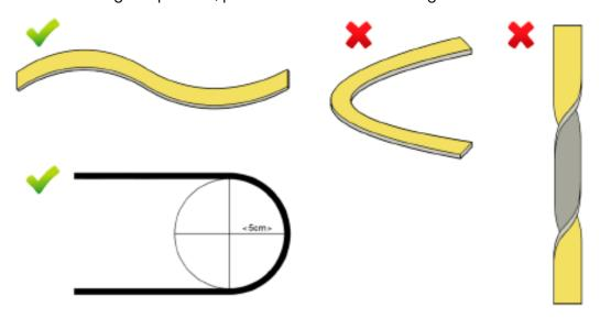
Cable and connector should never be stretched. Also, the LED strip should not be twisted. The LED strip is completely encapsulated and designed for versatile Use. It can be mounted in different ways and works equally well horizontally as vertically.
