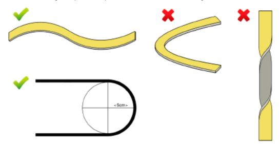
Cable and connector should never be stretched. Also, the LED strip should not be twisted. The LED strip is completely encapsulated and designed for versatile Use. It can be mounted in different ways and works equally well horizontally as vertically. When mounting the LED strip, It is important that the encapsulation is kept intact. We recommend use of the following types of mounting equipment:
