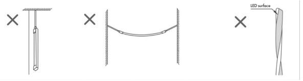
The LED strip is completely encapsulated and designed for versatile Use. It can be mounted in different ways and works equally well horizontally as vertically. When mounting the LED strip, it is important that the encapsulation is kept intact. We recommend use of the following types of mounting equipment:
