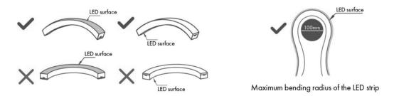
Cable and connector should never be stretched. Also, the LED strip should not be twisted.
